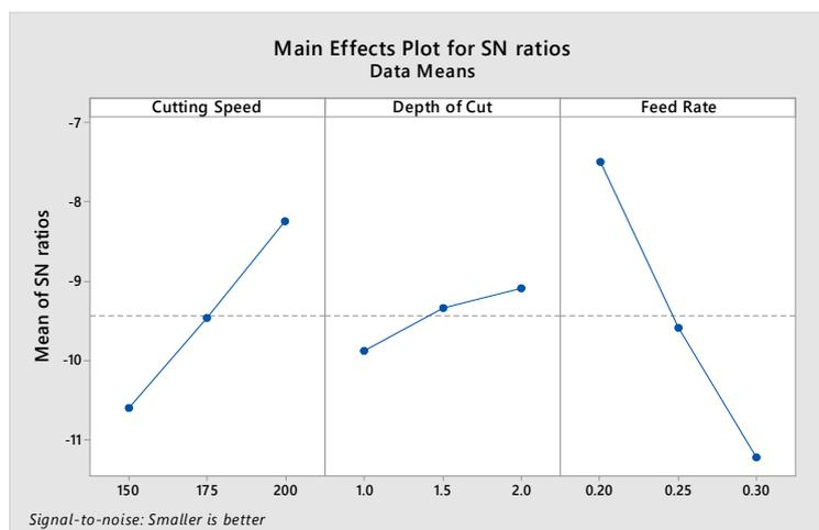
**Figure 5.5: Main effects plot for SN ratios for EN 31**
