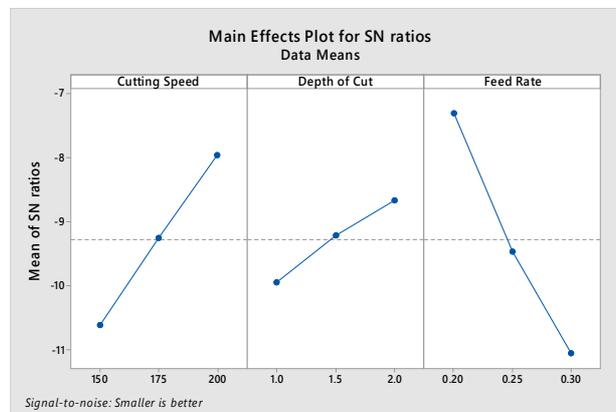
Figure 5.2: Main effects plot for SN ratios for EN 24
