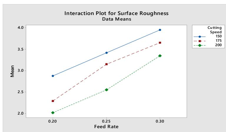
**Figure 5.6: Interaction plot for Surface Roughness for cutting speed vs feed rate for EN 31**
