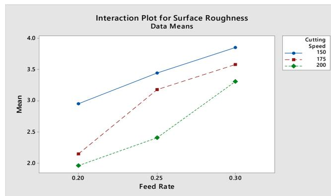
Figure 5.3: Interaction plot for Surface Roughness for cutting speed vs feed rate for EN 24
