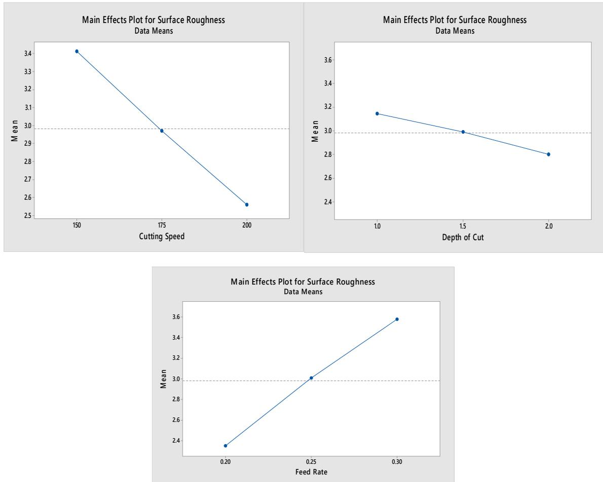
Figure 5.1: Main effects plot for Surface Roughness versus input parameters for EN 24
