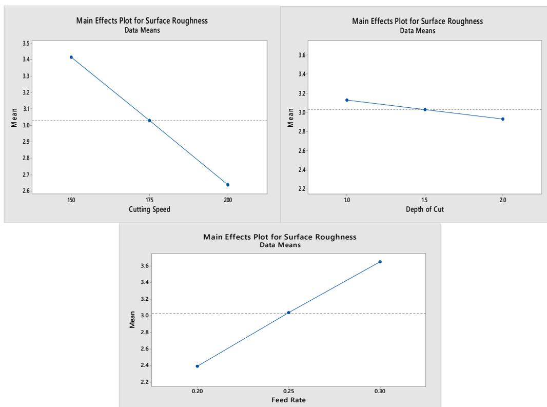
Figure 5.4: Main effects plot for Surface Roughness verses input parameters for EN 31
